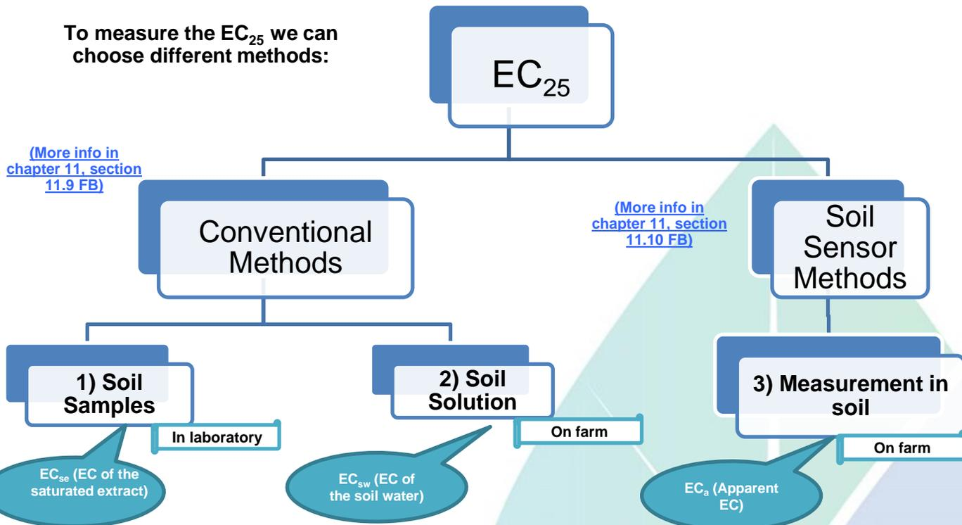
Normally 2) and 3) require several permanent sampling devices, which disrupt the soil's initial state. Because of this, it is advisable to wait for a few months after installation before data can be accepted as reliable.
