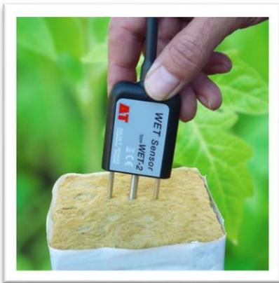
Reflectometry sensor used to take measurements on rockwool substrate (<https://www.delta-t.co.uk>)
