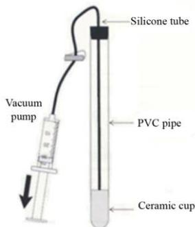
Diagram of a soil solution suction sampler
